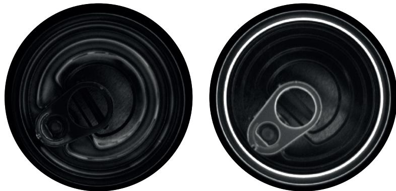
SACMI's Double Shot technology, allows the system to capture two images of the same object, under different lighting and in just under a millisecond. It is mainly applied on MVS systems for inspection of post-repair varnish on EOE lids (Double Shot UV).
